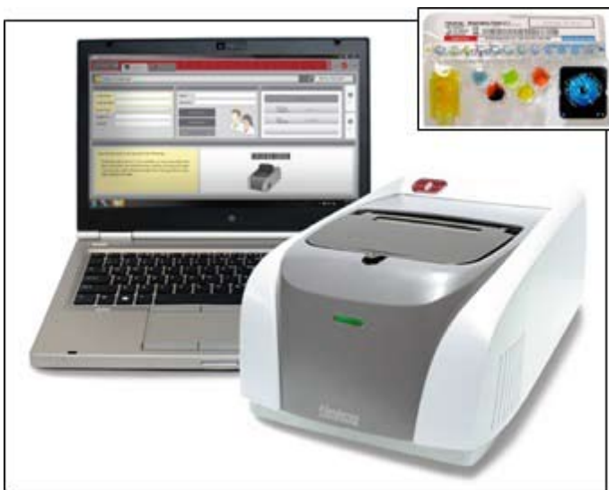
Figure 1. The FilmArray and the Respiratory Panel pouch with a laptop for analyzing results. (Images from the BioFire FilmArray EZ Configuration Operators Manual).
